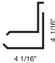
Wall Flashing and Under Wall Flashing
