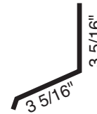
Wall Flashing No Return
